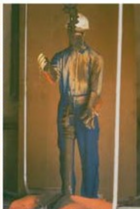
After Electric Arc Blast
