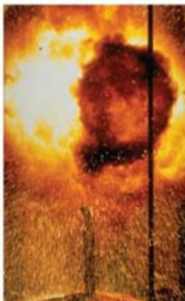
During Electric Arc Blast
