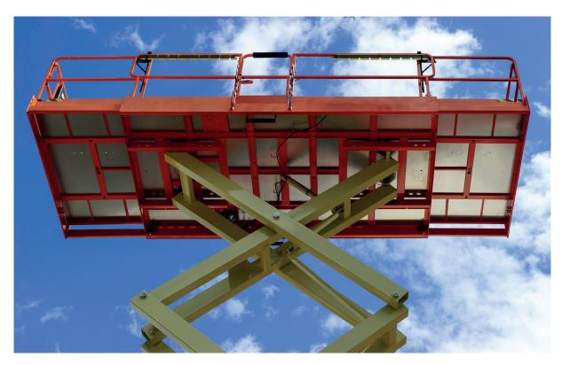
This alert has been generated to ensure that all sites in Australia are aware of the risks associated with the danger to workers of being crushed against structures, while manoeuvring raised mobile elevated work platforms (EWPs) and scissor lifts in, around or near fixed structures.
