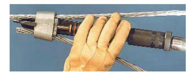
It has been brought to the attention of the ETU that some Electrical Distribution Companies and associated contractors are utilising an AMPACT shell fired tool to install conductor taps or stirrups. This alert has been developed to ensure that all of the hazards with this system are recognised.
