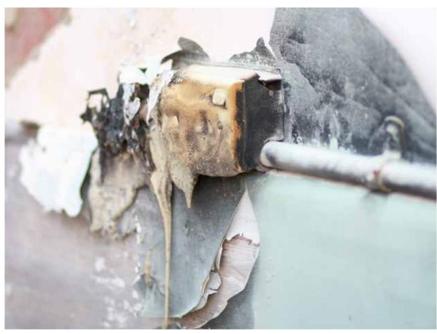
It appears that there was a fundamental design flaw when the pins on 3 pin plug tops were narrowed to allow for insulating medium to be installed to provide protection against inadvertent contact.
